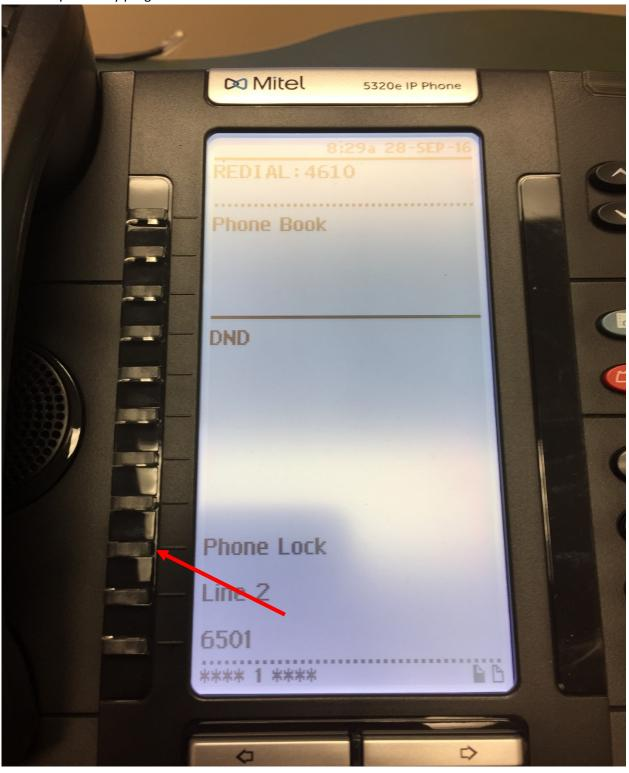
2. Your phone should now display LOCKED at the top of the screen and the Phone Lock button should be illuminated. All phone features are now LOCKED with the exception of Emergency Calls (911).
